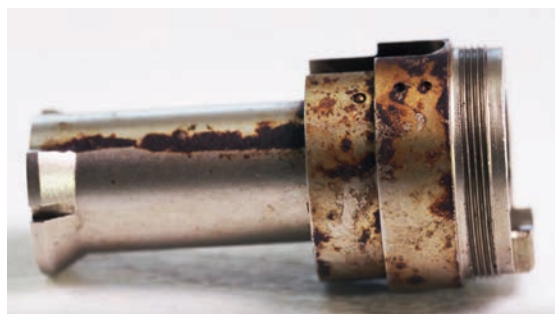
Fig. 1: Dental handpiece coupling with rust.
