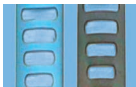
Section – titan valves: Lefthand valve – brand new. Righthand valve – washer disinfectant cleaned.
