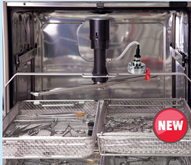
Fig. 1: EBI 12-TP237 temperature/pressure data logger in use in a washer-disinfector.
