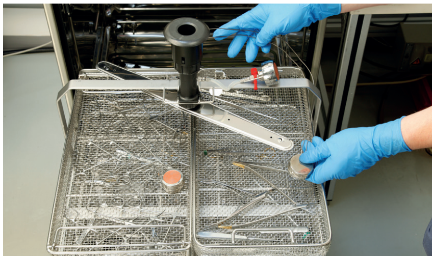
Fig. 2: Pressure measurement during washer-disinfector process validation.
