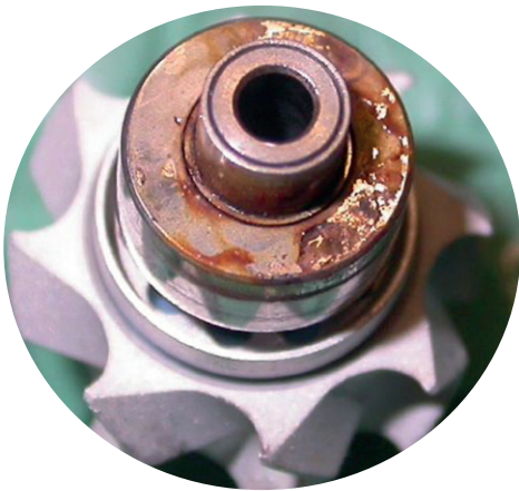
Fig. 3: Rotor of a dental turbine with rust-coloured deposits due to inadequate oiling.
