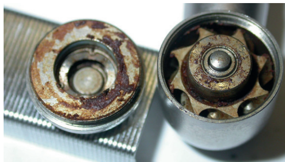
Fig. 2: Dental turbine with push button removed – rotor with residual soiling.
